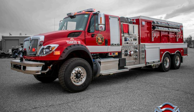
Boise Mobile Equipment's Tandem Axle Tender is the solution to your water delivery challenges. Tank options include stainless steel or poly with capacities up to 4,000 gallons for high water delivery. Pump configurations range from 250 GPM to 2,250 GPM, enabling responders to make the most of their tender, whether using it for tactical purposes or delivering water.
